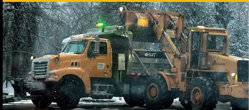
Since 2022, highway maintenance vehicles may display flashing green lights in work zones. These lights are different than regular amber lights and are used to signify that a work zone is upcoming.
